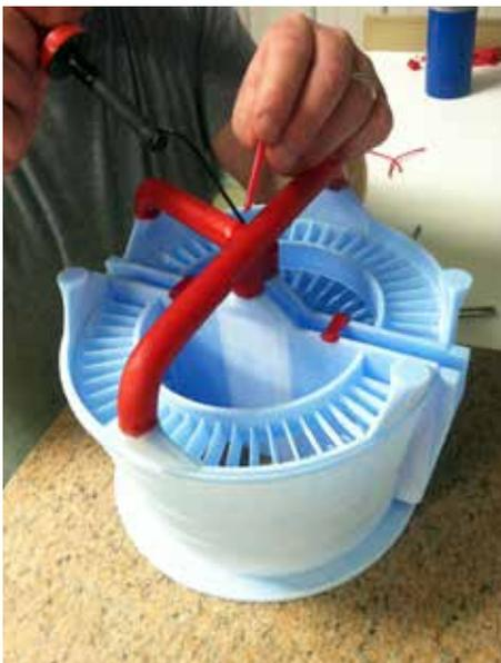
*Full casting pattern of stator case.*
